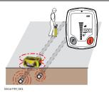
2. To confirm that the transmitter and the locator are on the same utility, place the signal transmitter upright and directly over the utility.
