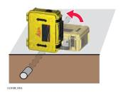
3. If the transmitter and the locater are on the same utility, the Numeric Peak Indicator on the locator significantly decreases.
