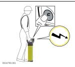
Ensure that the locator is held upright and close to the ground. Take care not to swing the locator.
