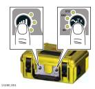
6. Set the locator to the required Signal Transmitter frequency.
